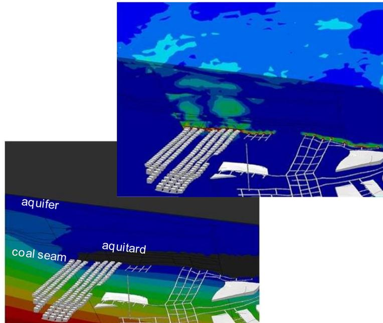
Coal mining induced damage distribution (upper) and pore pressure profile (lower).
